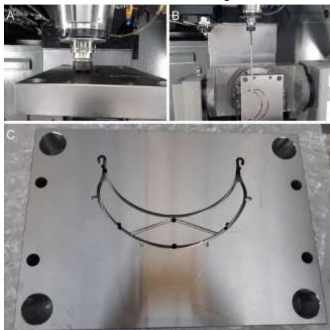
Figure 3 : Mold imprint fabricated at the Arts et Métiers campus of Bordeaux. A, B : machining steps. C: final imprint for injection
