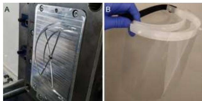
Figure 4 : Head band model by injection, produced at the Cachan IUT. A final imprint of the production mold. B fully functional face shield
