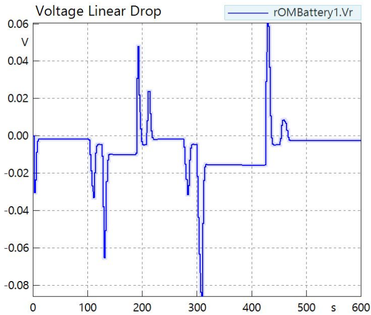
Figure 7.27 – Voltage drop produced by the internal resistance in a cell during the simulated. itinerary
