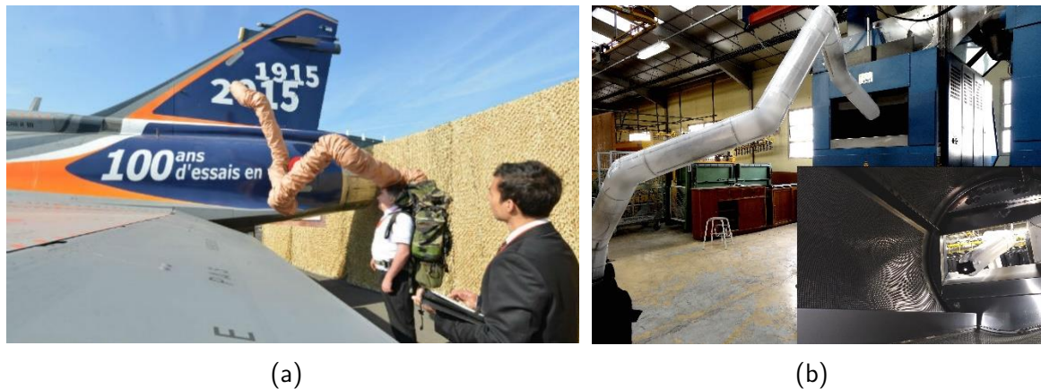
Figure 1.7 Demonstration of the Ultralight inflatable arm. (a) Inspection of an aircraft fuselage. (b) Inspection in an industrial environment.
