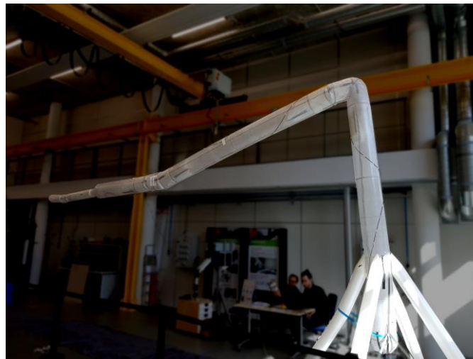
Figure 2.18 Prototype of the Ultra-lightweight inflatable arm. Its total length is 10 m, it has 6 degrees of freedom, a cross-section diameter of 30 cm. The last segment with a smaller diameter can be detached to modulate the total length.
